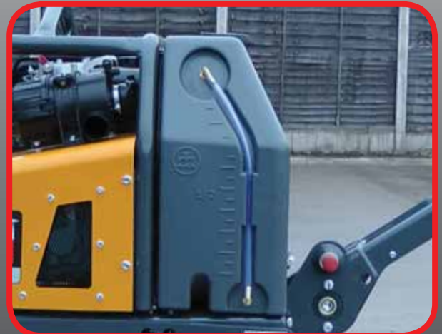
65ltr Water Tank with External Gauge
